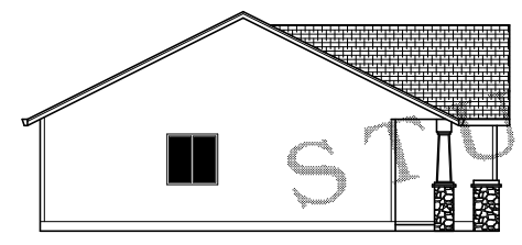
LEFT SIDE ELEVATION SCALE 1/8"=1'0"
